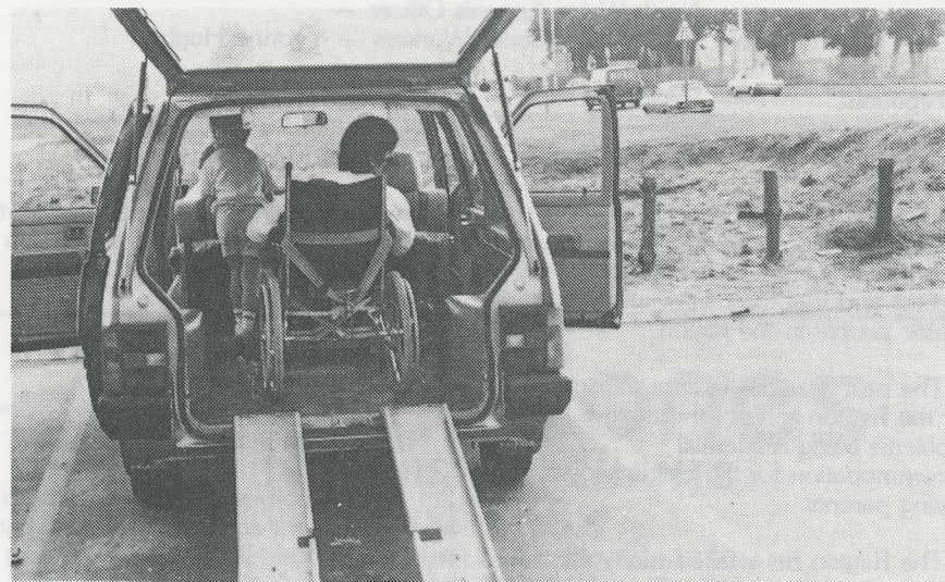
The photographs illustrate a DATSUN PRAIRIE which has been adapted to take a wheelchair with the occupant of the wheelchair clamped down in complete safety and having an excellent view.
